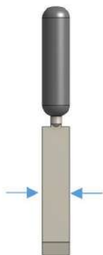
PRISE TOOL MIN WIDTH= 25MM
